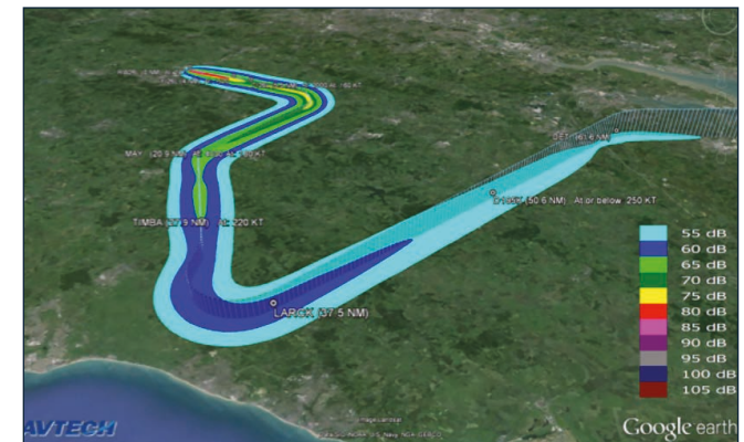
Figure 3 Runway 26 baseline example of an arrival from the east
